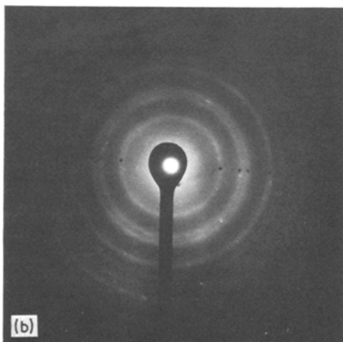
Figure 3 (a) Diffraction pattern of new metastable rhombohedral phase obtained in liquid-quenched and vapour-quenched antimony films. (b) Unidentified structure obtained on heating amorphous phase or (a). (c) Equilibrium rhombohedral phase obtained on heating (a) or (b).
